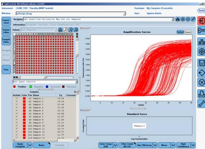
Figure 9. Obtaining the Crossing Point (Cp) Cycle values at the Second Derivative Maximum.
