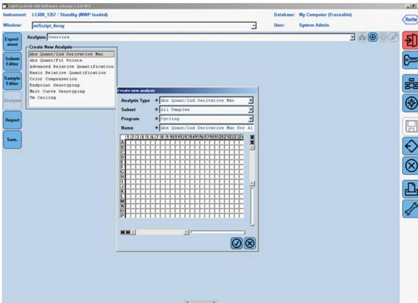
Figure 8. Setting up the analysis for the Second Derivative Maximum.
