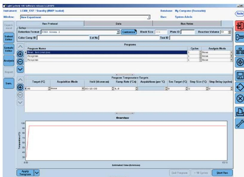
Figure 3. Setup for the first program — Heat Activation.
