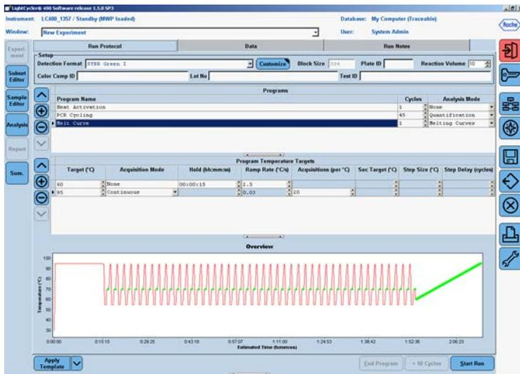
Figure 5. Setup of the third program — Melt Curve.
