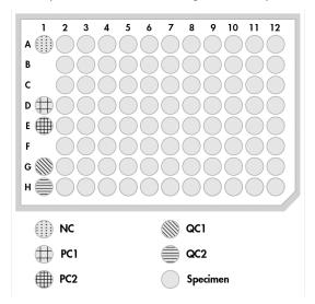
The RCS pipets the calibrators and quality controls into column 1 of the hybridization microplate. On the hybridization microplate, the RCS places the NC replicates in A1, B1, C1; the PC replicates in D1, E1, F1; the QC1 in G1; and the QC2 in H1.
