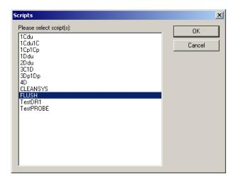
Repeat the FLUSH script until large bubbles are no longer seen in the lines or in the syringes.
