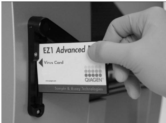
**Figure 1. Ease of protocol setup using EZ1 DSP Cards.** Inserting an EZ1 Card, preprogrammed with the protocol, into the EZ1 instrument.
