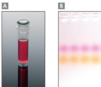
**Figure 1. Ready-to-load PCR products.** CoralLoad Dye **A** contains gel-tracking dyes **B** enabling immediate gel loading of PCR and easy visualization of DNA migration.
