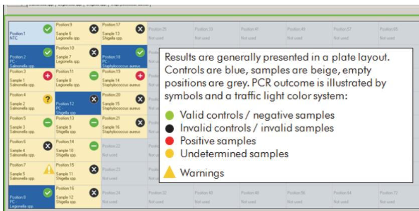
**Figure 4. An example of a Results Table (in software version 2.3).** The symbols are added to the results table, indicating the absence of the pathogen (green symbol), the presence of the pathogen (red symbol), undetermined samples (yellow symbol), or invalid samples (black symbols). The black and yellow symbols indicate that user attention is required.
