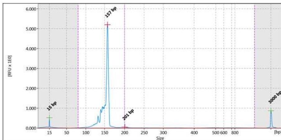
**Figure 4.** Trace data from the QIAxcel Advanced capillary electrophoresis instrument, showing the pooled and purified multiplex PCR product of the GeneRead QIAact BRCA1/2 Panel. A peak observed at approximately 157 bp represents the amplicons.
