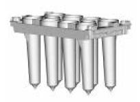
8-Rod-Covers cover the magnetic rods of the magnetic head.
