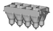
Purification of nucleic acids takes place in sample prep cartridges.
