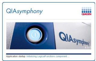
4. The QIAsymphony SP/AS instruments initialize. During initialization, the instruments carry out a self-test routine to check that the electronics and mechanics are functioning properly.
