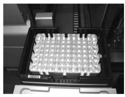
Adapter placed onto the transfer frame on slot 1 of the "Eluate" drawer.
