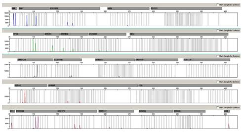
Figure 5. Electropherogram of STR analysis in the presence of degraded DNA (fragments of 150 bp). Genomic DNA was sheared to fragments of 150 bp using ultrasound. The large STR fragments were amplified with a very low PCR yield, but QS1 and QS2 were amplified normally with equal peak heights. The markers are shown at the top of the electropherogram. The Quality Sensors are labeled with BTP (panel 5) and appear at fragment sizes of 74 bp (QS1) and 435 bp (QS2).
