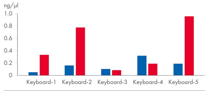
**Figure 6. Keyboard: Concentration of DNA (ng/μl) recovered from surface swabs by processing with AutoMate Express and EZ2 Connect Fx.**
