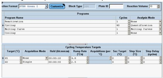
4. Select "Melting Curve" and set up the parameters for melting curve analysis as shown below. Be sure to select "Continuous" for "Acquisition Mode" at the 95°C step.
