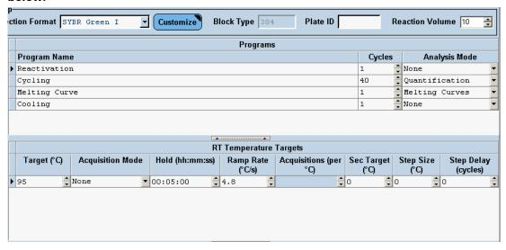
3. Select "Cycling" and set up the parameters for PCR cycling as shown below. Be sure to select "Single" for "Acquisition Mode" at the 60°C step.
