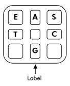
**Figure 2. Illustration of the PyroMark Q24 Cartridge seen from above.** The annotations correspond to the label on the reagent vials. Add enzyme mixture (**E**), substrate mixture (**S**), and nucleotides (**A**, **T**, **C**, **G**) according to the volume information given in the Pre Run information report, found in the "Tools" menu at run setup.
