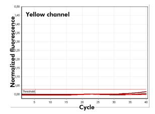
**Figure 3. The PCR is inhibited**. There is no amplification of the three samples in the green channel (left) or the internal control in the yellow channel (right). All curves lie along the baseline and do not exceed a preset threshold.
