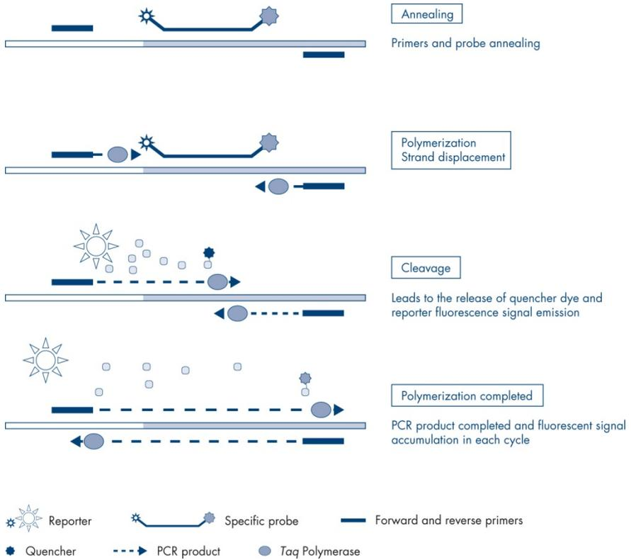
**Figure 3. Principle of TaqMan real-time PCR assay.**
