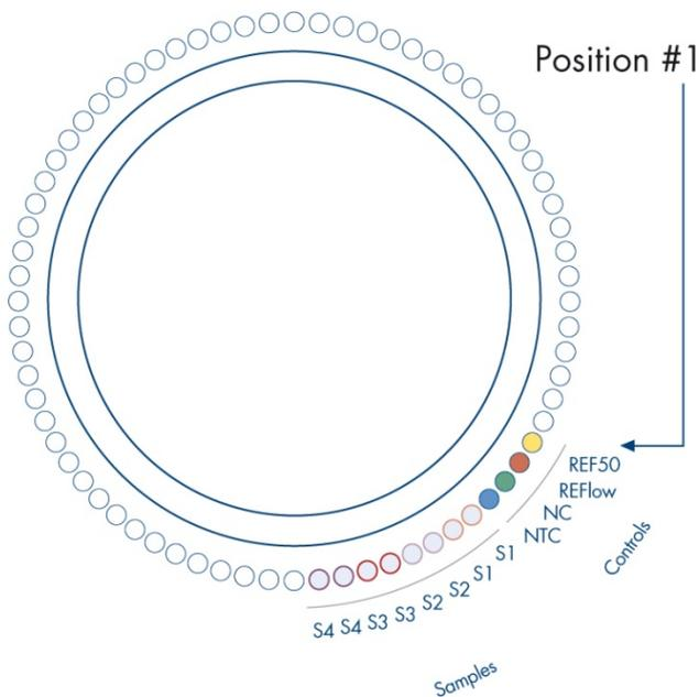
**Figure 5. Rotor setup for an experiment with the *thetascreen* PITX2 RGQ PCR Kit. REF50:** PITX2 RGQ PCR Reference 50; **REFlow:** PITX2 RGQ PCR Reference Low; **NC:** PITX2 RGQ PCR Negative Control, **NTC:** PITX2 RGQ PCR NTC (NTC); **S1 to S4:** bisDNA samples. **Note:** All of the remaining positions ○ should be filled with empty tubes.
