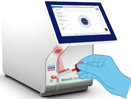
Figure 11. Scanning sample ID bar code.
