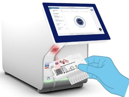
Figure 12. Scanning QIAstat-Dx Viral Vesicular Panel Cartridge bar code.
