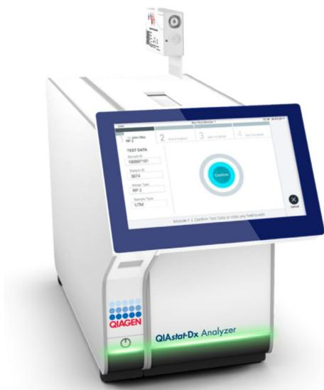
**Figure 14. Inserting QIAstat-Dx Viral Vesicular Panel Cartridge into QIAstat-Dx Analyzer 1.0.**
