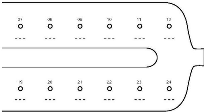
Figure 3. Labeling scheme for tubes and QIAamp Mini columns for use on the QIAvac 24 Plus vacuum system
