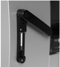
Figure 2. Complete insertion of EZ1 Card. The EZ1 Card must be completely inserted before the EZ1 instrument is switched on.
