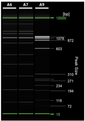
Figure 8. Recovery of small DNA fragments. A6: Ladder after purification using the 300 µl protocol. A7: Equivalent amount before extraction. A9: QIAxcel DNA size standard.
