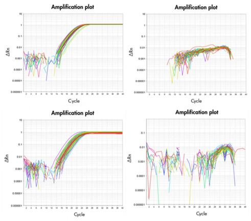
**Figure 11. Contamination study with the 500 µl protocol.** Eluates from buccal swab samples (left) and negative samples (right) were quantified using the Investigator Quantiplex HYres Kit on an Applied Biosystems 7500 Real-Time PCR System for Human Identification.
