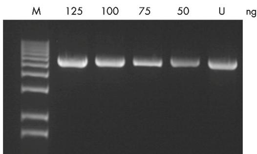
**Figure 4. Agarose gel analysis.** An unknown amount of a 5.5 kb DNA fragment (**U**) was run alongside known quantities (as indicated in ng) of the same DNA fragment. The unknown sample contained 75–100 ng DNA, as estimated by visual comparison with the standards. **M**: 1 kb DNA ladder.
