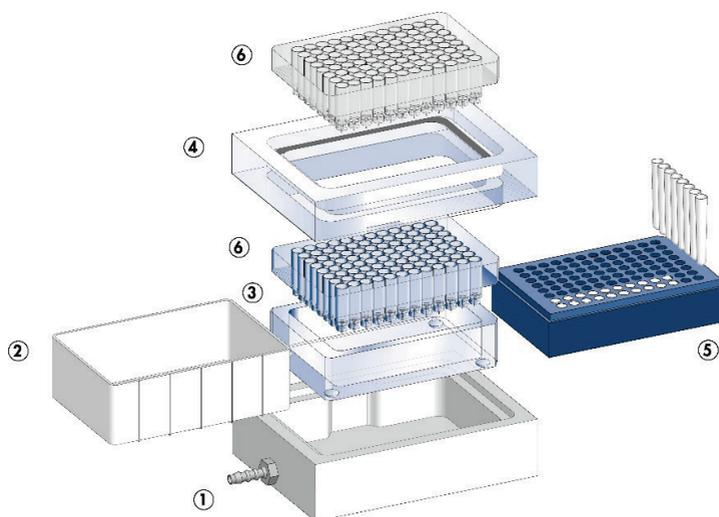
**Figure 6. Components of the QIAvac 96 manifold.** 1: QIAvac base, which holds a waste tray, a plate holder, or a microtube rack. 2: Waste tray. 3: Plate holder (shown with 96-well plate) 4: QIAvac 96 top plate with aperture for 96-well plate. 5: Microtube rack. 6: 96-well plate (not included with QIAvac 96, included in QIAprep 96 Turbo Miniprep Kits)
