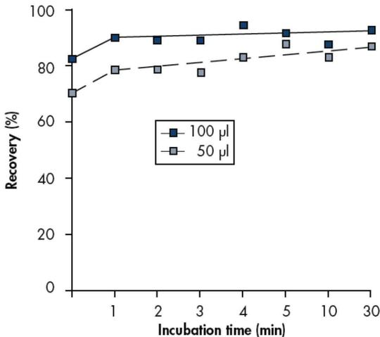
**Figure 3. Incubation time versus DNA recovery.** Using the QIAprep Spin Miniprep protocol, 10 μg pBluescript® DNA was purified and eluted after the indicated incubation times with either 50 μl or 100 μl Buffer EB. The graph shows that an incubation time of 1 minute and doubling the elution buffer volume increase yield.
