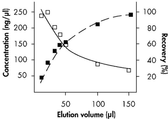
**Figure 2. Elution volume versus DNA concentration and recovery.** Using the QIAprep Spin protocol, 10 μg pUC18 DNA was purified and eluted with the indicated volumes of Buffer EB. The standard protocol uses 50 μl Buffer EB for elution, because this combines high yield with high concentration. However the yield can be increased by increasing the elution volume.
