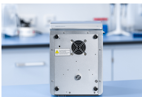
Figure 24. QIAmini with transport lock screw in transport position.
