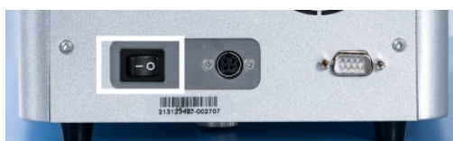
Figure 5. Location of the power switch (highlighted with a white frame).
