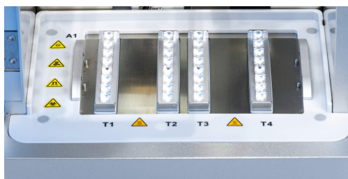
Figure 9. The heater block of QIAmini consists of four rows (T1, T2, T3, and T4).
