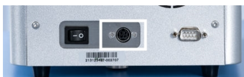
Figure 6. Location of the power cord socket (highlighted with a white frame).
