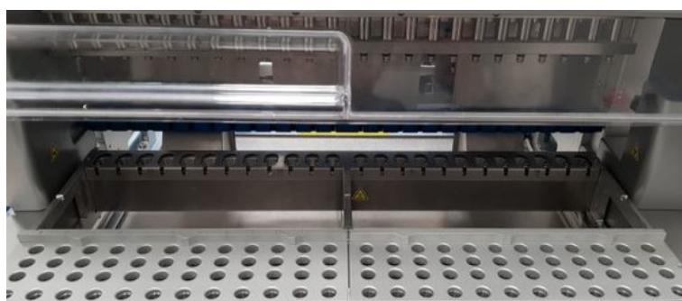
Figure 14. Tip rack with four inserted tip holders/filter tips.
