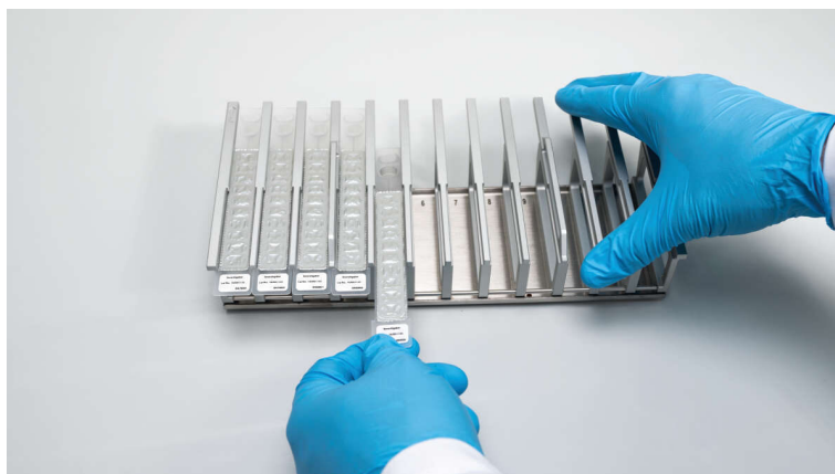
Figure 11. Cartridge rack with some cartridges inserted.
