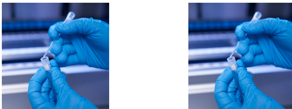
Figure 187. Preparation of filter tips for grease application.
