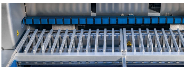
Figure 12. Removable cartridge rack inside the instrument.
