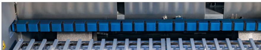
Figure 19. The EZ2 Connect MDx magnet module.
