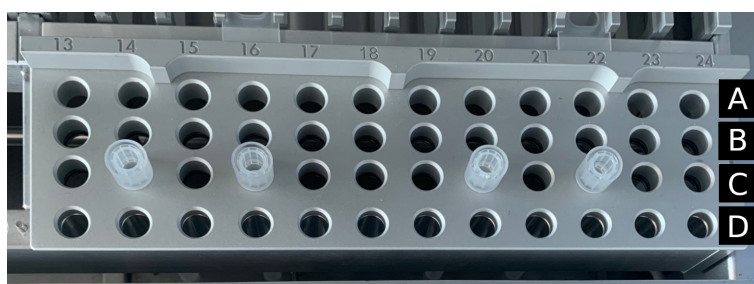
Figure 14. Tip rack with four inserted tip holders/filter tips.
