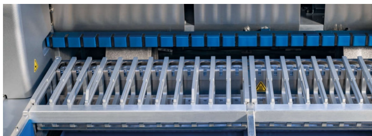
Figure 12. Removable cartridge rack inside the instrument.
