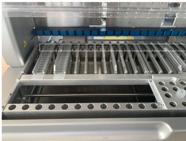
Figure 17. Heatable positions in the cartridge rack (highlighted by white frame).
