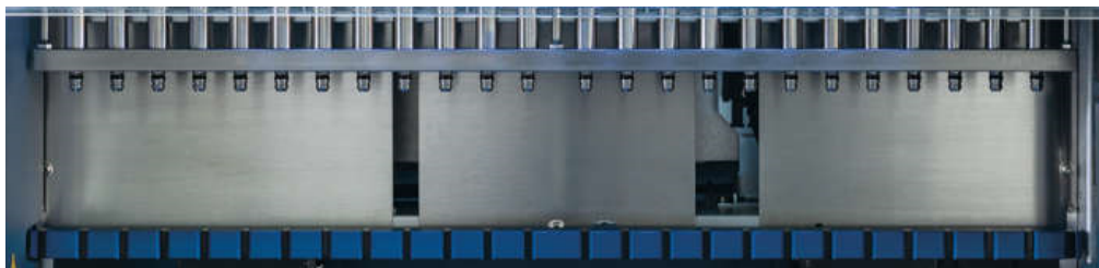
Figure 10. EZ2 Connect MDx pipettor head.
