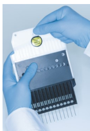
Figure 1. Removal of purge cap seal.
