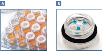
Figure 1 A EasyXtal Pre-Screen Assay 24-well plate and B DropGuard Crystallization Support.
