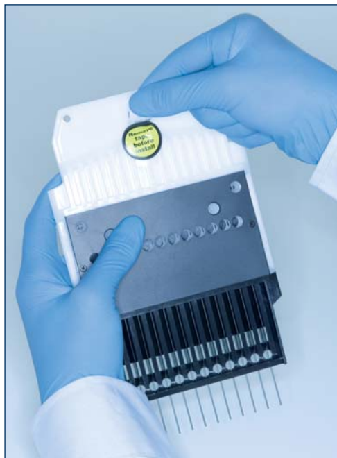
Preparing the QIAxcel Gel Cartridge.
