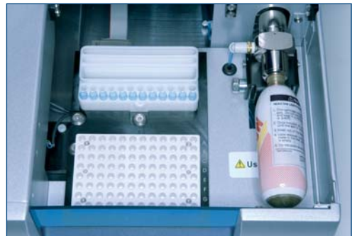
Loading the buffer tray.
