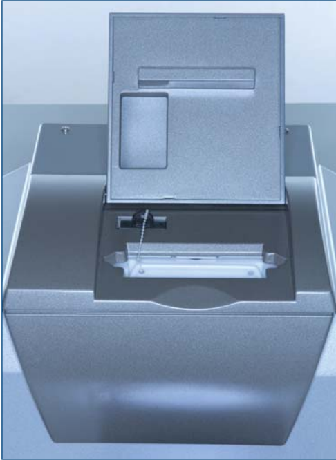
Installing the QIAxcel Gel Cartridge and smart key.
