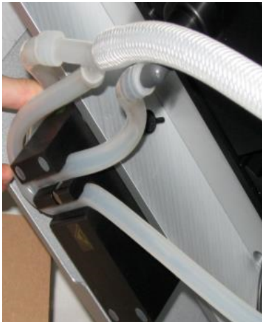
Hose exiting from the pinch valve.
