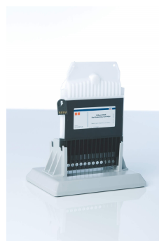
Figure 2. Preparing the QIAxcel gel cartridge. Upright storage in QX Cartridge Stand (cat. no. 929708) is recommended.
