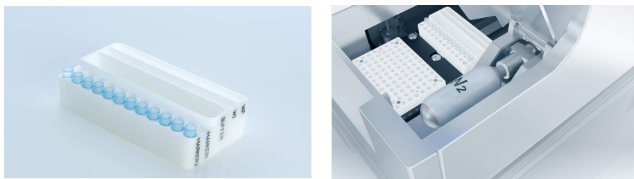
Figure 3. Preparing the buffer tray and inserting the buffer tray into the buffer tray holder.
