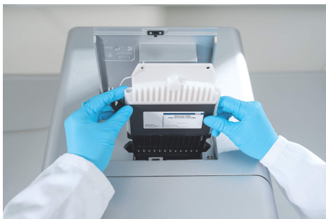
Figure 4. Installing the QIAxcel gel cartridge and smart key in the QIAxcel instrument.
