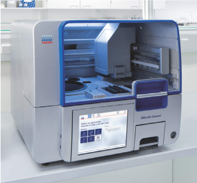
Figure 2. Fully automated spin-column based nucleic acid purification. The QIAcube Connect enables walkaway automation of many QIAGEN spin-column procedures. Visit www.qiagen.com/MyQIAcubeConnect for more information.
