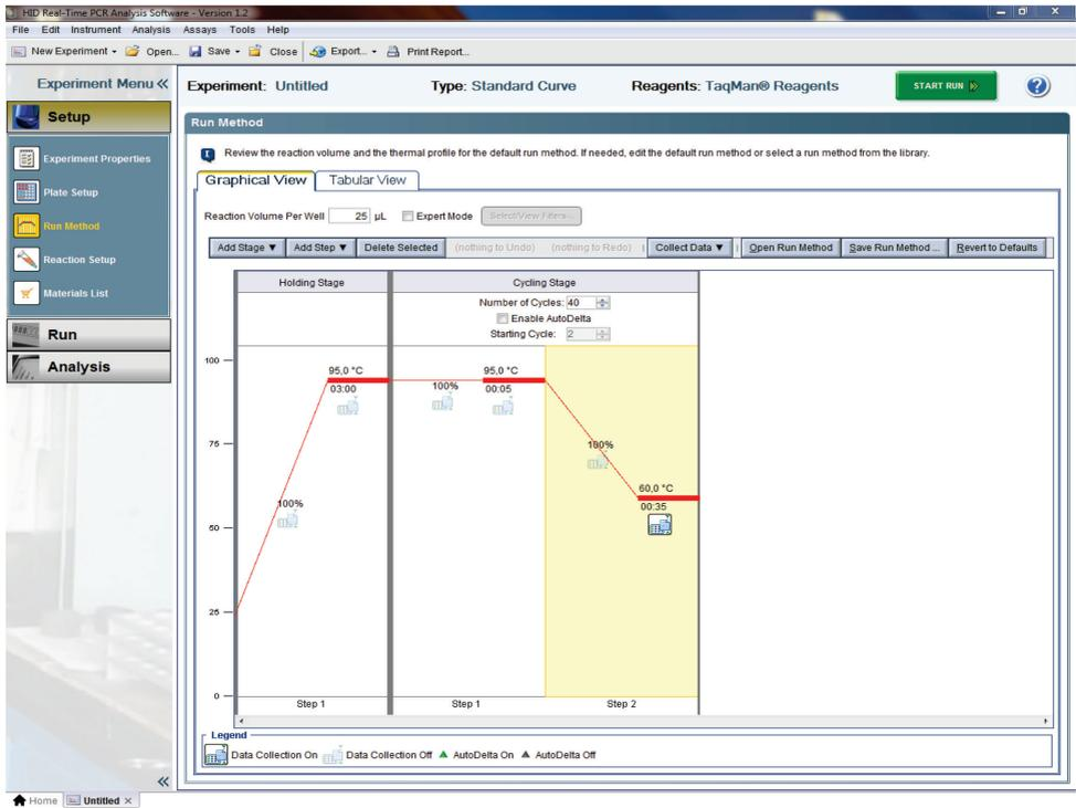
**Adjusting the thermal profile (HID Real-Time PCR Analysis Software v1.1 or v1.2).**
