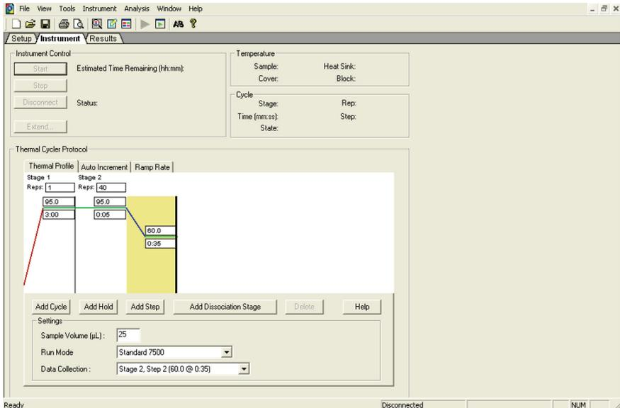
**Adjusting the thermal profile (SDS Software Version 1.4).**
