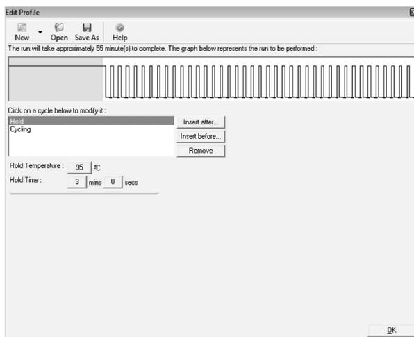
**Initial PCR activation step. PCR requires an initial incubation at 95°C for 3 min to activate the DNA polymerase.**
