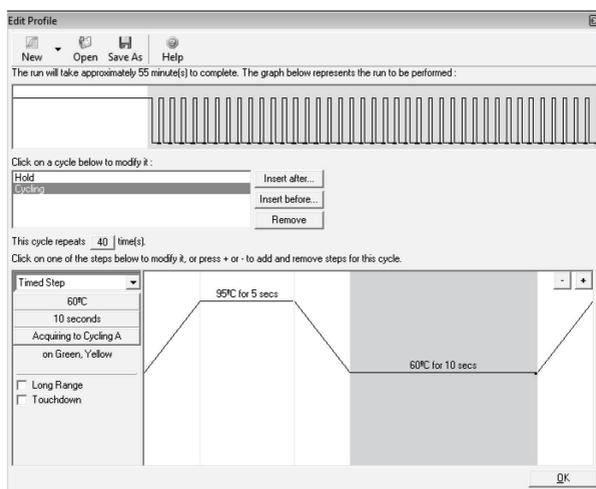
**Two-step cycling. PCR requires 40 cycles. Each cycle is comprised of 2 steps: 95°C for 5 s (denaturation step) and 60°C for 10 s (annealing/extension step).**
