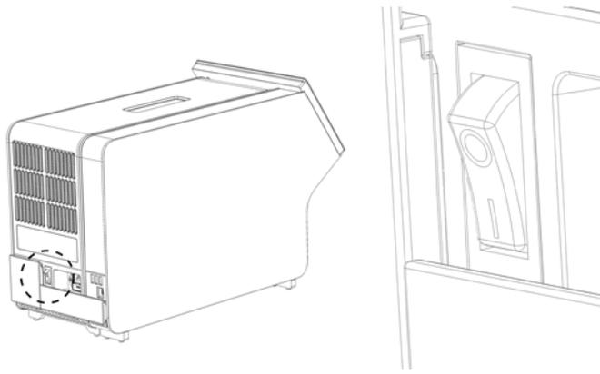
**Figure 21. Locating the power switch and setting it to the "I" position.**
