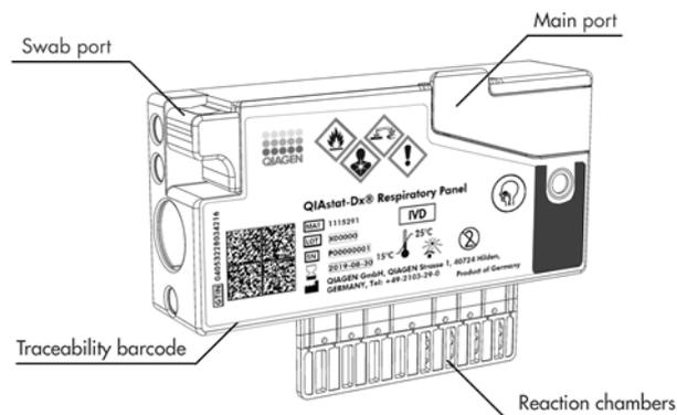
Figure 3. QIAstat-Dx assay cartridge features.
