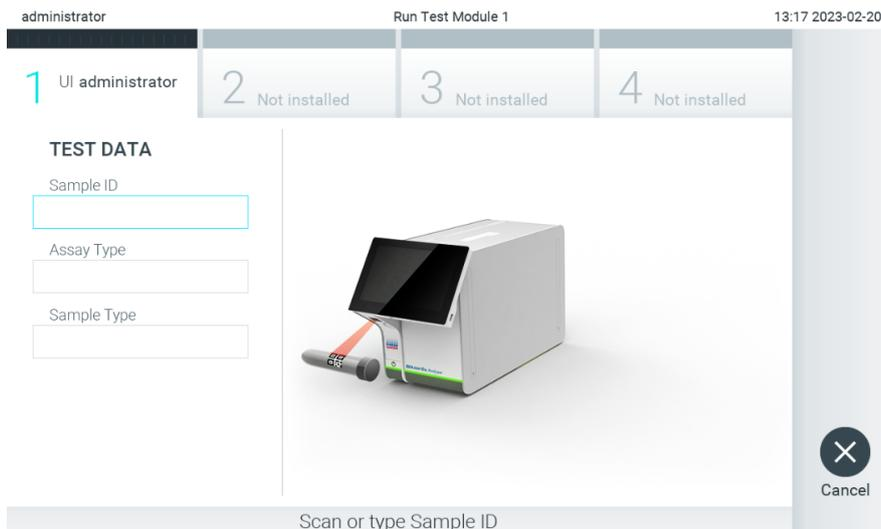
**Figure 85. Scanning the sample ID bar code**
