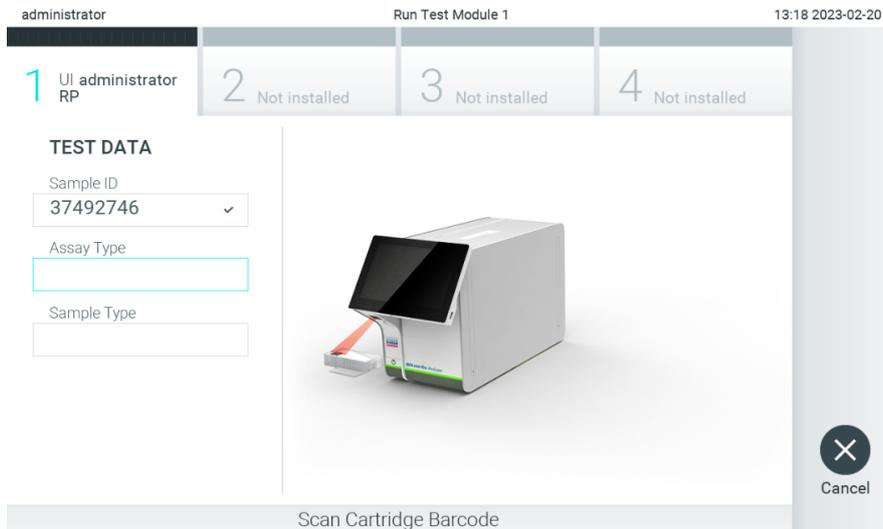
Figure 87. Scanning the QIAstat-Dx assay cartridge bar code.
