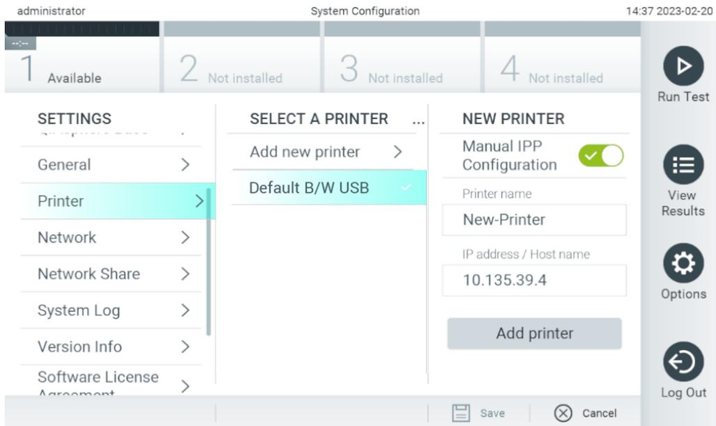
Figure 105. Printer installation with manual IPP configuration.
