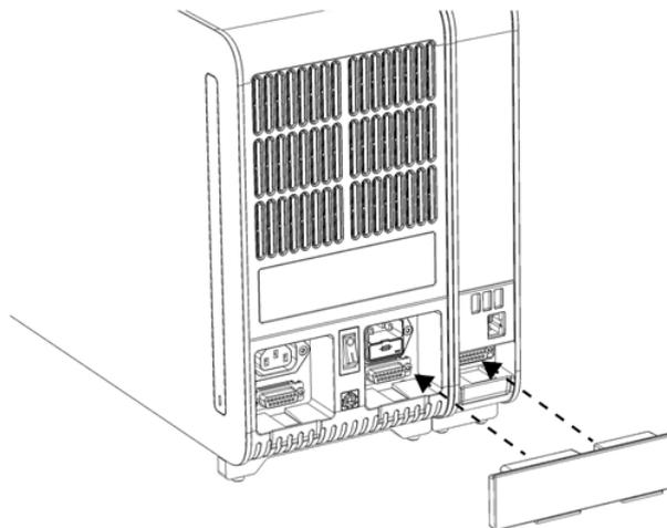
**Figure 8. Connecting the Analytical/Operational Module Bridge.**
