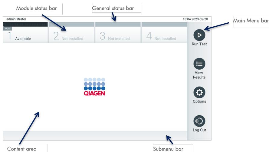
Figure 42. Main screen of the QIAstat-Dx Analyzer 2.0 touchscreen.
