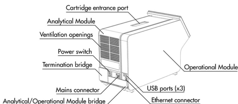
**Figure 2. Rear view of the QIAstat-Dx Analyzer 2.0.** The Operational Module is on the right and the Analytical Module is on the left.
