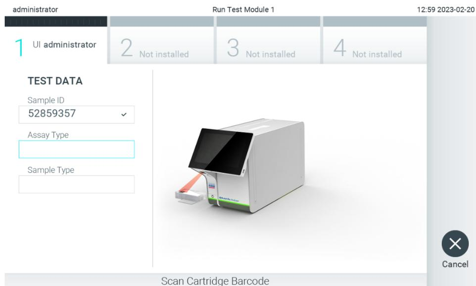
**Figure 24.** Scanning the QIAstat-Dx assay cartridge bar code.
