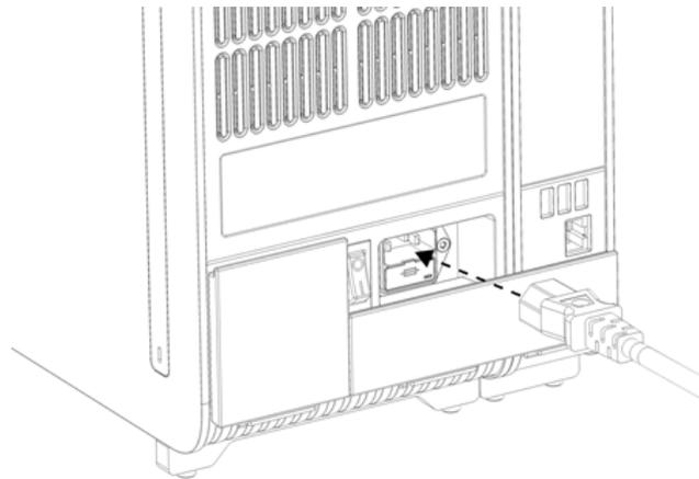
**Figure 20. Connecting the power cord.**
