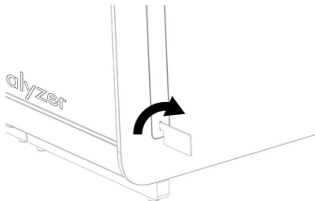
**Figure 15. Removing protective covers.**
