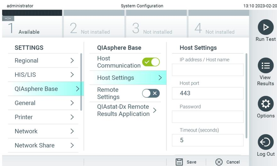
Figure 65. Configuring the QIASphere Base connection.
