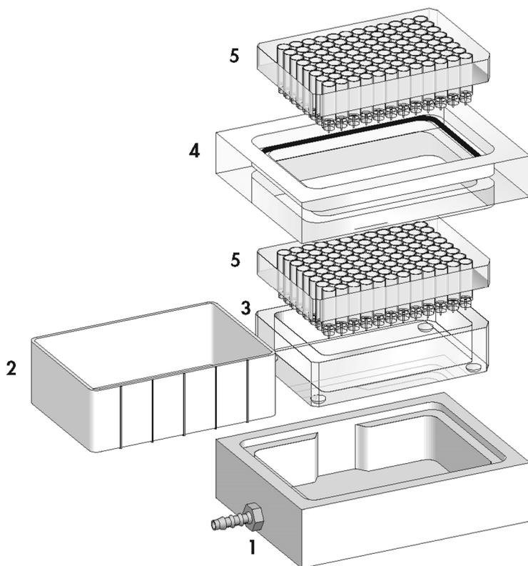
**Figure 1. Components of the QIAvac 96 vacuum manifold.**
