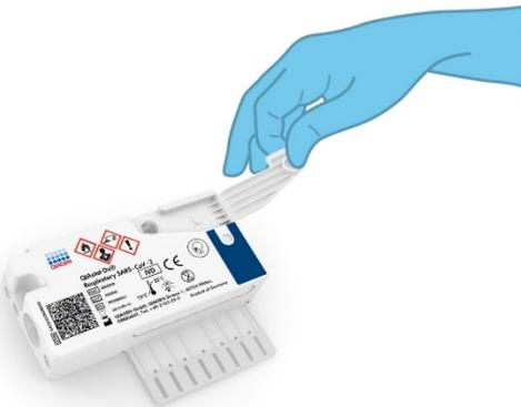
**Figure 39. Opening the sample lid of main port.**
