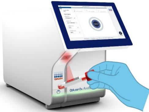
**Figure 44. Scanning sample ID bar code.**
