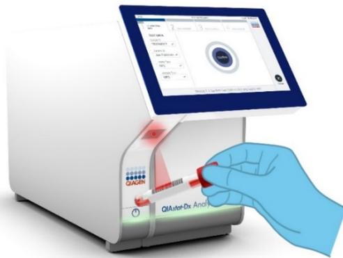
**Figure 11. Scanning sample ID bar code.**
