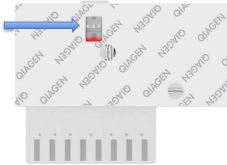
Figure 43. Sample inspection window (blue arrow).
