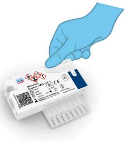
**Figure 42. Closing the sample lid of the main port.**
