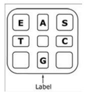
**Figure 4. Illustration of the PyroMark Q24 Cartridge, as seen from above.** The annotations correspond to the label on the reagent vials. Add enzyme mixture (**E**), substrate mixture (**S**), and nucleotides (**A**, **T**, **C**, **G**) according to the volume information given in the Pre Run information report, found in the "Tools" menu at run setup.
