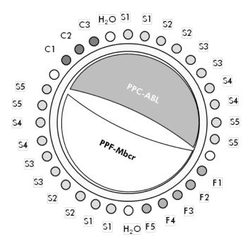
Figure 5. Suggested rotor setup for each experiment with the *ipsogen* BCR-ABL1 Mbcr Kit. F1–5: BCR-ABL Mbcr standards; C1–3: ABL standards; S: unknown DNA sample to be analyzed; H<sub>2</sub>O: water control.
