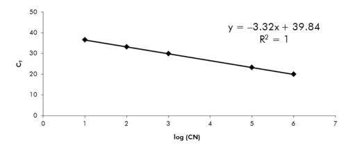
Figure 9. Theoretical curve calculated from the 5 standard dilutions. A linear regression curve (y = ax + b) is calculated for each gene (ABL and BCR-ABL), where a is the slope of the line and b is the y-intercept, which is the y-coordinate of the point where the line crosses the y axis. Its equation and coefficient of determination ( $R^2$ ) are printed on the graph.
