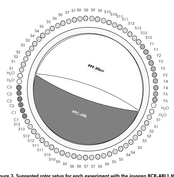
Figure 3. Suggested rotor setup for each experiment with the *ipsogen* BCR-ABL1 Mbcr Kit. F1–5: BCR-ABL Mbcr standards; C1–3: ABL standards; S: cDNA sample; H<sub>2</sub>O: water control.
