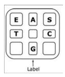
**Figure 5. Illustration of the PyroMark Q24 Cartridge as seen from above.** The annotations correspond to the label on the reagent vials. Add enzyme mixture (**E**), substrate mixture (**S**), and nucleotides (**A, T, C, G**) according to the volume information given in the Pre Run information report found in the "Tools" menu at run setup.
