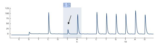
Figure 10. Pyrogram trace obtained after analysis of samples with a GTG  $\rightarrow$  GAG (V600E) mutation in base 2 of codon 600 (nucleotide 1799, indicated with an arrow) with "Sequence to Analyze" CWCTGTAGC.
