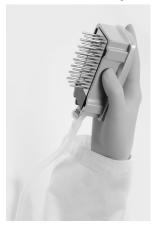
Figure 4. Illustration of the vacuum tool raised to beyond 90° vertical.
