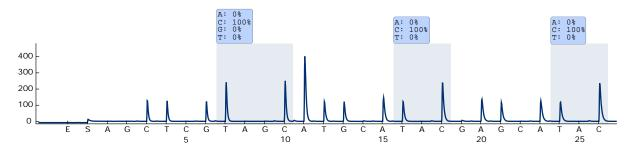
Figure 9. Pyrogram trace obtained after analysis of a sample with a wild type genotype in codons 464–469 with "Sequence to Analyze" CTGTTNCAAATGATHCAGATHCA.
