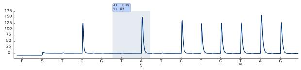
Figure 8. Pyrogram trace obtained after analysis of a sample with a wild type genotype in codon 600 with "Sequence to Analyze" CWCTGTAGC.
