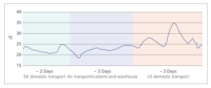
Figure 3. Temperature during Summer Transport of whole blood samples collected into PAXgene Blood ccfDNA Tubes (CE-IVD) from QIAGEN (Hilden, Germany) to BD (Franklin Lakes, USA).
