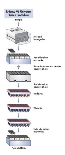
RNA purification with the RNeasy 96 Universal Tissue Kit. Protocol steps can be performed in a specially designed centrifuge system (page 13) with optional use of the QIAvac 96 vacuum manifold (page 14).
