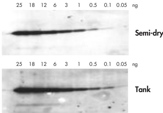
**Figure 7.** The indicated amounts of purified 6xHis-tagged DHFR mixed with crude extract from HeLa cells (8 µg total protein) were applied to an SDS-polyacrylamide gel. Western blots were prepared in an electrophoretic transfer apparatus according to the method indicated. 6xHis-tagged protein was detected with Penta-His Antibody diluted 1/2000 followed by HRP-conjugated rabbit anti-mouse IgG and ECL™ detection system.
