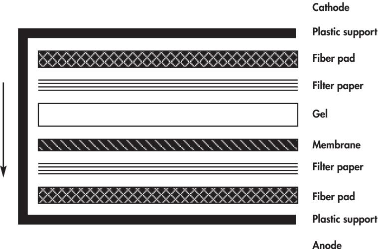
**Figure 10.** Schematic drawing of indicated blotting methods. Arrows show direction of transfer.
