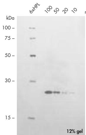
**Figure 11.** The indicated amounts of purified 6xHis-tagged DHFR mixed with crude extract from E. coli cells (8 µg total protein per lane) were applied to a 12% SDS-polyacrylamide gel. After electrophoresis and western transfer, 6xHis-tagged proteins were detected with Penta-His Antibody followed by chromogenic detection with AP-conjugated rabbit anti-mouse IgG and NBT/BCIP detection reagent. **6xHPL:** 6xHis Protein Ladder (2.5 µl).
