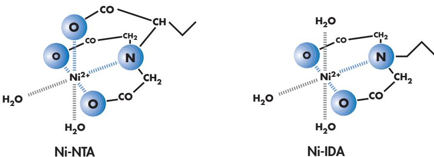
**Figure 2.** Comparison of the interactions of different metal chelate matrices with nickel ions.
