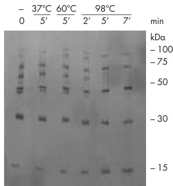
**Figure 9.** Effect of insufficient heating. The 6xHis Protein Ladder was dissolved as described above and heated at different temperatures for the different times shown. After electrophoresis and western transfer, 6xHis-tagged proteins were detected using Penta-His Antibody followed by AP-conjugated anti-mouse antibody and chromogenic substrate (BCIP/NBT).
