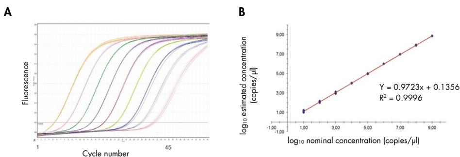
**Figure 10.** Amplification curve (A) and linear regression analysis (B) of a dilution series of genomic DNA from HAdV-2 (species C).
