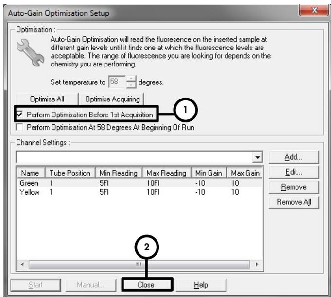
Figure 7. Adjusting the fluorescence channel sensitivity.
