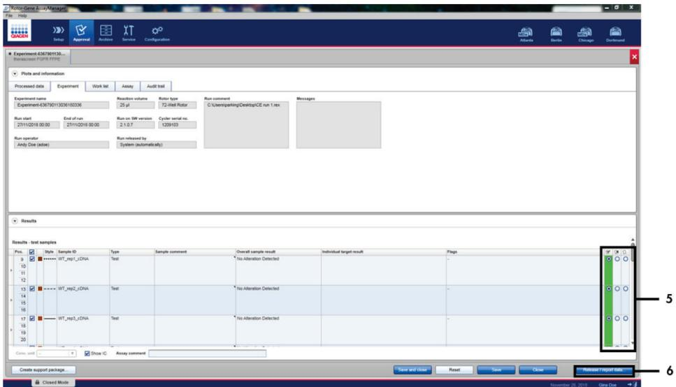
**Figure 16. Example of assay results main windows.** 1 = "Experiment" tab. 2 = "Plots and information" area. 3 = "Results" area. 4 = "Release/report data". 5 = Accept or reject radio buttons. 6 = Release/report data.
