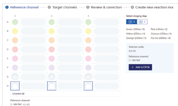
Figure 1. First step of generating a custom cross talk matrix. The well/s containing master mix are selected.
