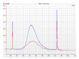
Figure 5: Capillary electrophoresis device trace of generated libraries. Capillary electrophoresis device trace data showing the correct size distribution of completed libraries and the absence of adapters or adapter dimers. Red line: library without/before enrichment. Blue line: same library after PCR enrichment.
