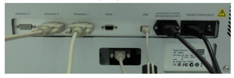
12.Connect one end of the AC power cord (standard 3-wire IEC mains cable) to the power connector of the vacuum control station. Connect the other end to the AC power outlet.
