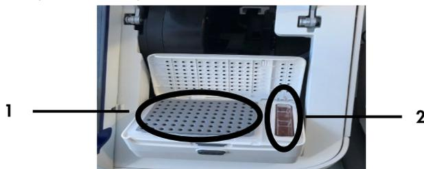
Figure 3. Plate holder and cathode buffer holder. 1 – Plate holder; 2 – Cathode buffer holder.
