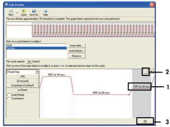
Figure 28. Removal of the extension step. 1 = Third step; 2 = Delete; 3 = "OK."
