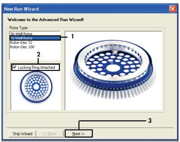
Figure 33. The "New Run Wizard" dialog box and welcome screen. 1 = "Rotor type"; 2 = "Locking Ring Attached" box; 3 = "Next."
