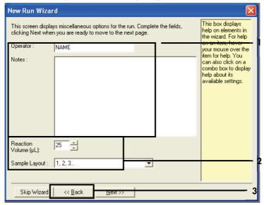
Figure 21. Entering operator name and reaction volumes. 1 = "Operator" dialog field and "Notes" dialog field; 2 = "Reaction Volume" field and "Sample Layout" field; 3 = "Next."
