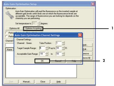
Figure 30. Auto-gain optimization for the Green channel. 1 = "Optimize Acquiring"; 2 = "OK."
