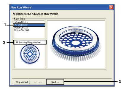
Figure 20. The "New Run Wizard" dialog box. 1 = "Rotor type"; 2 = "Locking Ring Attached" box; 3 = "Next."
