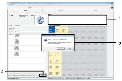
Figure 5. "Notes" field (1), "Start Run" button (2) and "Warning" of unused rotor positions (3).
