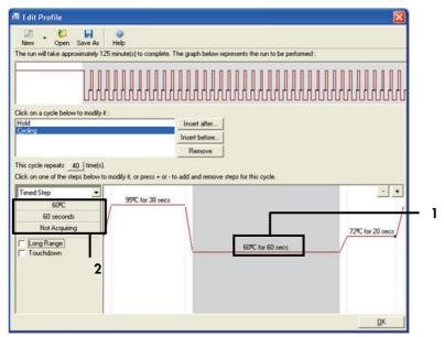
Figure 26. Cycling step at 60°C. 1 = Step two: temperature and time setting; 2 = "Not Acquiring."
