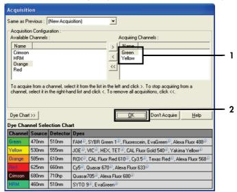
Figure 27. Acquiring at cycling step of 60°C. 1 = Selected channels; 2 = "OK."
