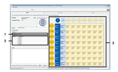
**Figure 13. Entering additional sample names in the "Sample Name" field.** 1 = "Sample Name" field; 2 = "Sample List"; 3 = "Layout of the pipetting adaptor" panel.
