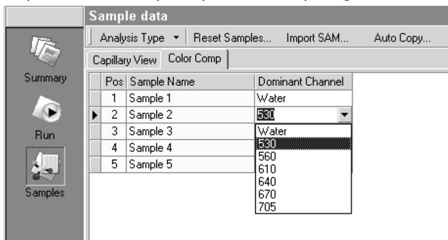
**Note:** *Sample 1* must be 2x master mix diluted with water to a 1x concentration (use the master mix supplied with the QuantiFast or QuantiTect Multiplex Kit). For *Sample 1*, the "Dominant Channel" must be set to *Water*. Be sure to set a different "Dominant Channel" for each sample.
