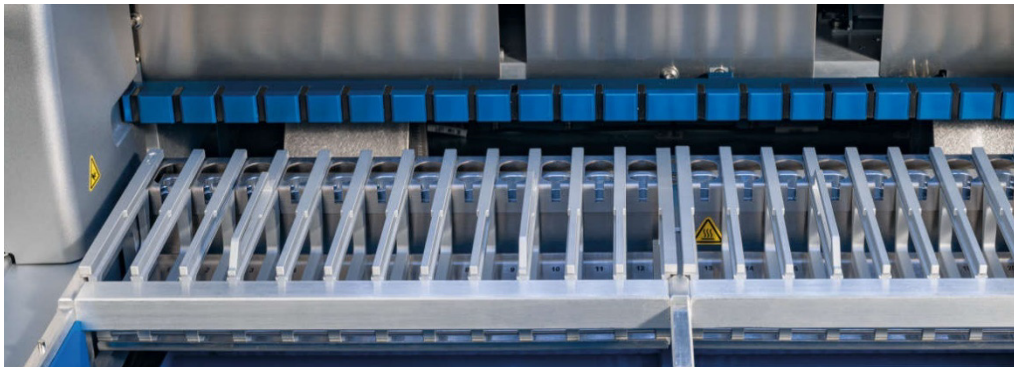
Figure 11. Removable cartridge rack inside the instrument.
