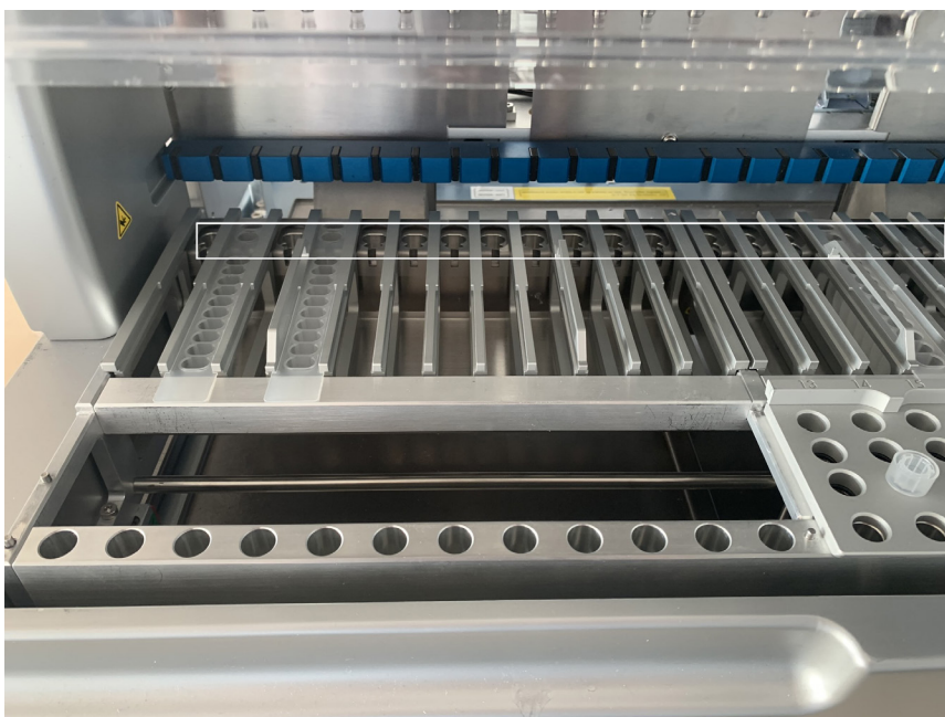
Figure 16. Heatable positions in the cartridge rack (marked by white frame).
