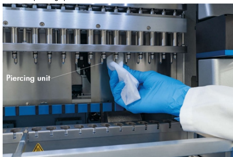
Figure 147. Cleaning the EZ2 piercing unit.
