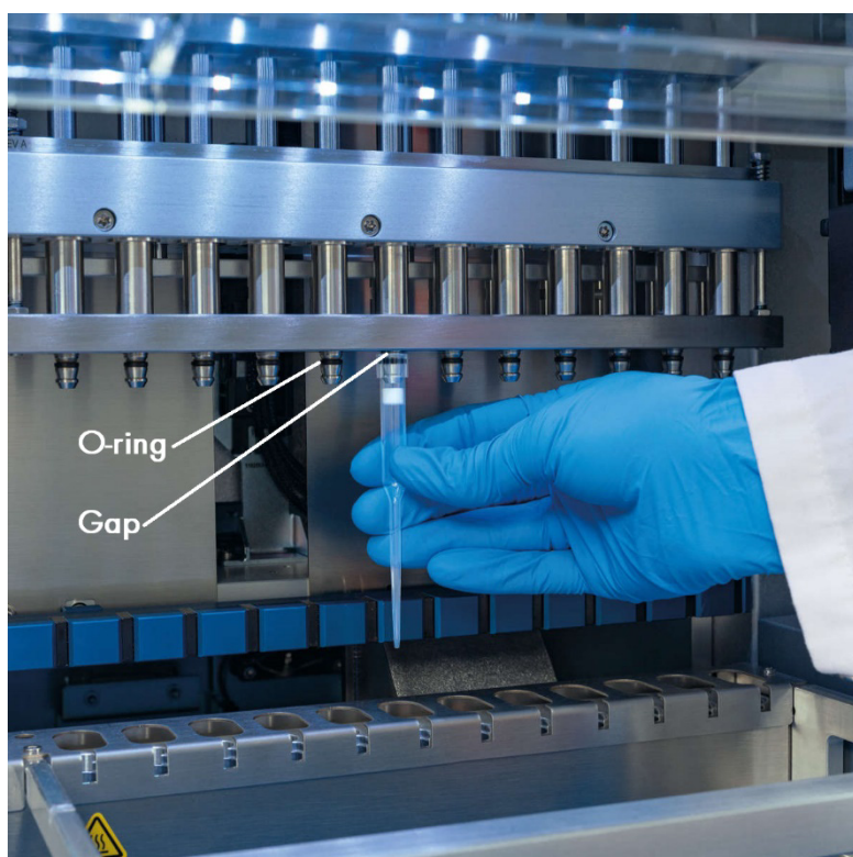
Figure 152. Placing a filter-tip onto the pipettor head.
