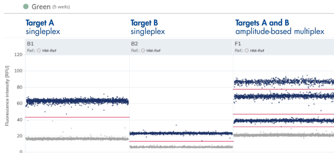
Figure 1. Example of 1D Scatterplots with amplitude-based multiplexing in QIAcuity Software Suite 3.1. Assays detecting 2 different targets (Targets A and B) were run in the Green channel. When run in singleplex reactions, assays for Target A (well B1) and Target B (well B2) each generate a single, sharp band of positive signal (dark blue). Because Target A was amplified with a higher concentration of assay compared to Target B, the amplitude of signal for Target A is greater than that for Target B. When the assays for targets A and B are combined in an amplitude-based multiplex reaction (well F1), 3 sharp clusters of clearly separated positive signal are generated. Using QIAcuity Software 3.1, multiple thresholds (red lines) can be set between these clusters. In the example shown in well F1, the lower cluster of signal corresponds to partitions positive for Target B only, while the middle cluster of signal corresponds to partitions positive for Target A only. The uppermost cluster corresponds to partitions positive for both targets A and B. Partitions negative for template are presented as gray signal.
