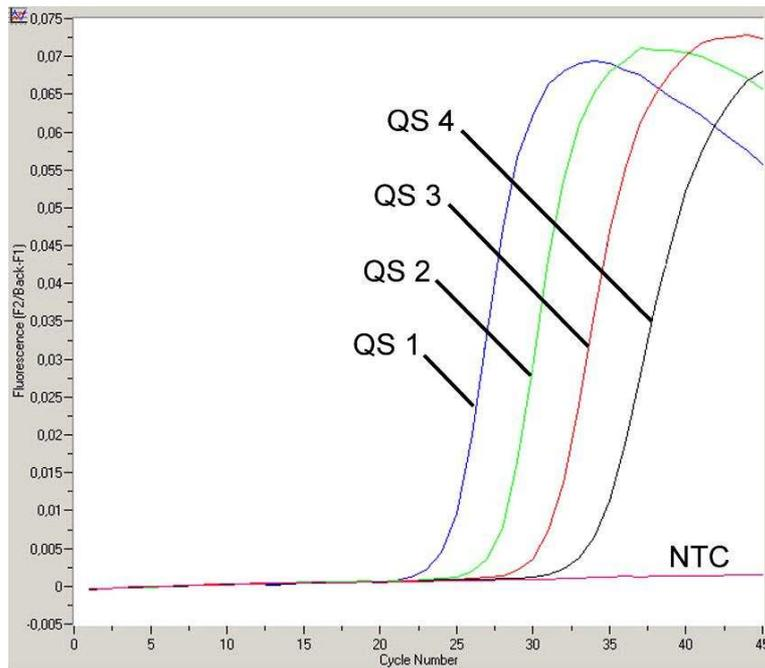
Fig. 7: Detection of the *Quantitation Standards (Orthopox LC QS 1 - 4)* in fluorimeter channel F2/Back-F1. NTC: non-template control (negative control).
