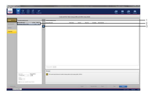
Figure 7. Setting up new manual worklist: Choosing assay profile name. 1 = "Assays" tab, 2 = Available assay profiles with "therascreen\_PIK3CA\_FFPE" or "therascreen\_PIK3CA\_Plasma" selected, 3 = Select the assay profile.
