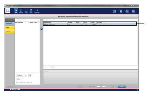
Figure 8. Create work list main window. 1 = Add the number of samples.
