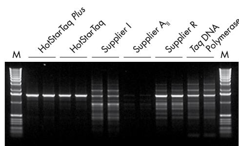
**Figure 1. Highest specificity with HotStarTaq Plus DNA Polymerase.** PCR was carried out using QIAGEN HotStarTaq Plus, HotStarTaq, and Taq DNA Polymerases and 3 hot-start PCR enzymes from the indicated suppliers. Parallel reactions were performed following the suppliers' recommendations, using 50 ng human genomic DNA. A 1.5 kb fragment of the human CFTR gene was amplified in 35 PCR cycles. Only QIAGEN hot-start enzymes provided highly specific amplification. **M:** markers.
