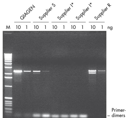
**Figure 5. Highly sensitive and reliable PCR.** PCR was carried out using HotStar HiFidelity DNA Polymerase (QIAGEN) and 4 high-fidelity PCR enzymes from the indicated suppliers. A 2.3 kb fragment of the human IL9R gene was amplified from differing amounts of genomic DNA in 40 PCR cycles. **M:** markers.
